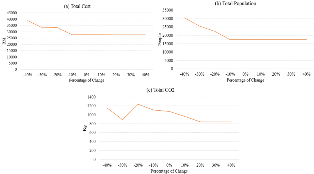
Figure 9: Effect of the collection facility capacity on the objective functions: (a) The first objective function. (b) The second objective function. (c) The third objective function.
